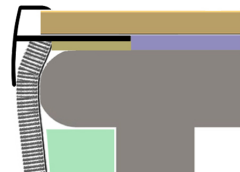
Top Nose fitted with 2mm MDF Strip, 4mm Underlay and Easyshim's to the riser
